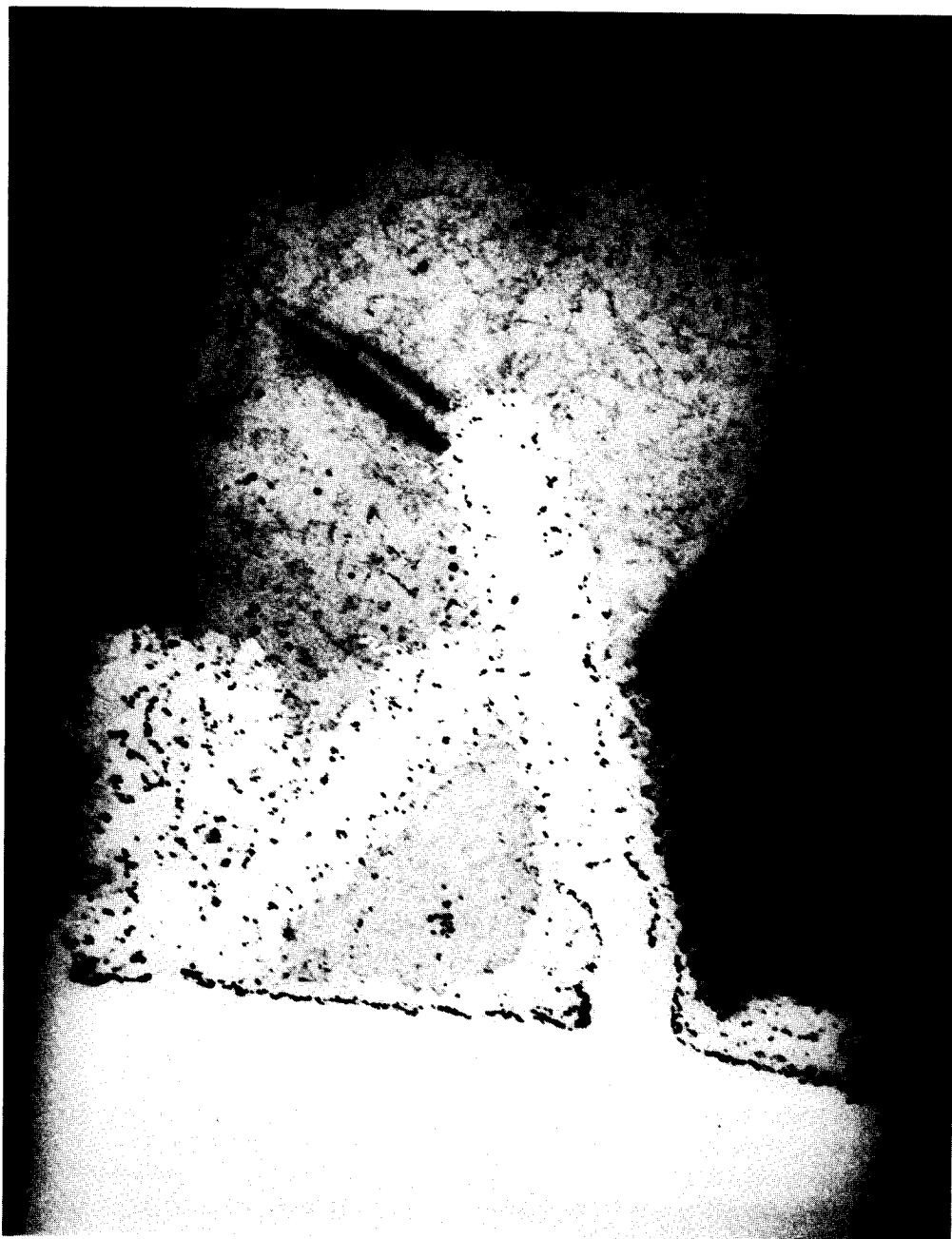
FIG. 6. Transmission micrograph showing both channel broadening by uncatalyzed attack and reformation of nickel particles on a sample which has been heated in 1 Torr hydrogen at 1200°C and then exposed to 5 Torr oxygen at 1065°C.
